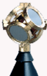
The SoundField multi-capsule mic array.
